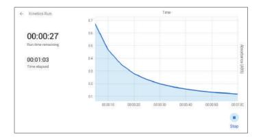
Once the measurement time is complete the results will be shown on the screen.
