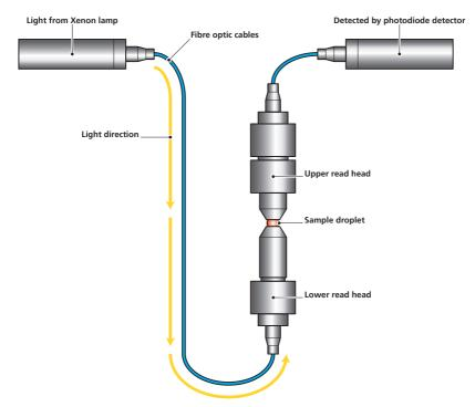
The optical layout of the SP-500-NANO spectrophotometer is shown below:
