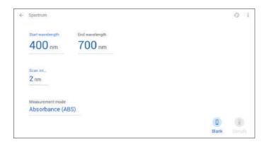
The start and end wavelengths must be different. If the same value is entered an error message will be displayed.
