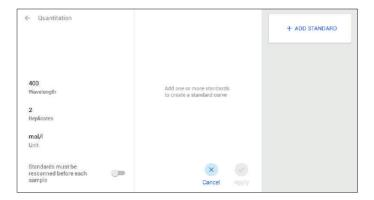
Touch  $\frac{100 \text{ mol/l}}{100 \text{ mol/l}}$  to use keypad to enter the concentration value required for that standard. Touch **Done** to apply.
