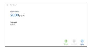
Touch  $\bigvee_{\text{Apply}}$  to save the absorbance result for the 1st standard.
