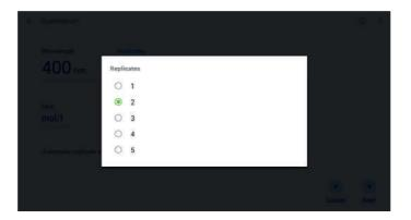
If 2 or more replicates are selected, Automatic replicates measurement becomes active. Automatic replicates will read the same sample for the selected number of replicates. If individual sample replicates are being used, do not select the automatic replicates option.
