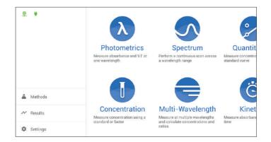
This spectrophotometer is controlled solely through the touchscreen interface of the equipment and follows a basic Android user interface. If the number of options available in a menu exceeds the number that can be displayed on the screen, swipe to the left to view the other modes.
