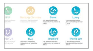
All of the five colorimetric protein assays modes are based on the Quantitation mode and differ only in the wavelength they use. They all have an option of a background correction wavelength if required by the protocol. See below for settings.
